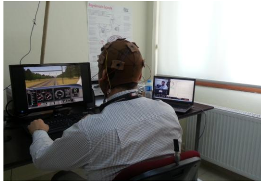
Figure 3. The organization of the virtual passive continuous control task used for testing the described EEG-BCI attention state detection system. In the experiments, participants engaged in controlling a simulated passenger train on a primarily featureless segment of track for the duration of 35 to 55 minutes.
