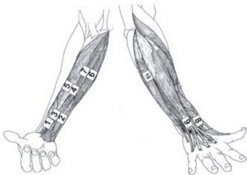
Figure 2. Possible electrode locations for surface EMG measurements as related to hand movements. Locations 3 and 4 have been used in this work.
