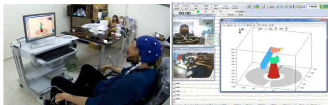
Fig. 7. Online experiments in which the participants have controlled a 3 dof-robot manipulator arm using EEG BCI.
